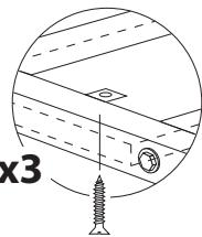
Place the drawer on the lower section of the workbench and screw the tabs to the shelf.
