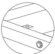
Locate the tabs located underneath the workbench.
