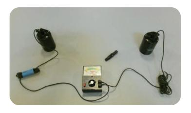
Press the red test button. The reading should be between 10^E6 to 10^E9. The reading below would be about 6x10^E8.
