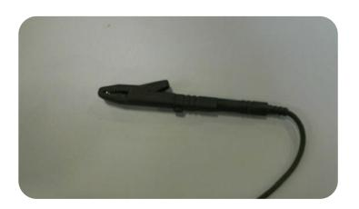
Attach the alligator clip to the ground stud under the top. You should still get the same reading as between the two weights on the surface. This verifies that the ground stud is conducting the electricity away from the top.
